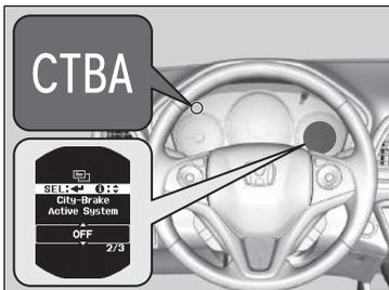
You can turn the system on and off using the multi-information display.
