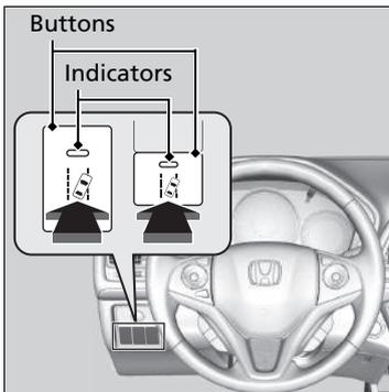
Press the Lane Departure Warning button to turn the system on and off.
