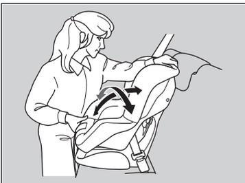
5. Push down the tab. Route the shoulder part of the belt into the slit at the side of the restraint.
