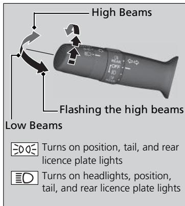
Rotating the light switch turns the lights on and off, regardless of the position of the ignition switch\*1.
