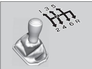
When you are not shifting, do not rest your foot on the clutch pedal. This can cause your clutch to wear out faster.
