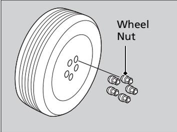
1. Remove the wheel nuts and flat tyre.
