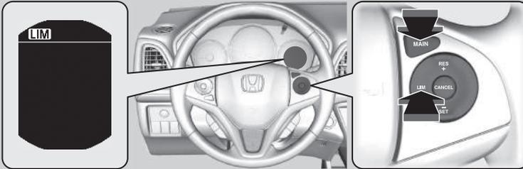
If a different indicator comes on, press the **LIM** button to switch to the adjustable speed limiter.
