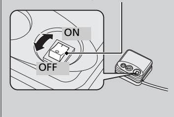
6. Plug in the compressor to the accessory power socket.
