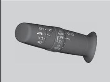
Automatic lighting control can be used when the ignition switch is in ON
