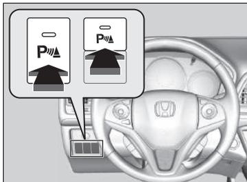
With the ignition switch in ON [II]<sup>\*1</sup>, press the parking sensor system button to turn on or off the system. The indicator in the button comes on when the system is on.
