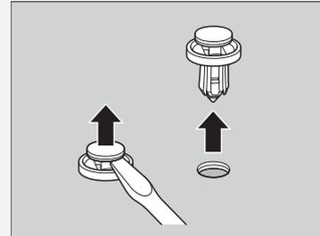
Insert the clip with the centre pin raised, and push until it is flat.
