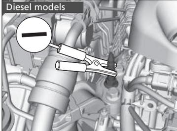
4. Connect the other end of the second jumper cable to the stud bolt as shown. Do not connect this jumper cable to any other part.
