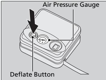
7. Turn the air compressor switch on to inflate the tyre.
