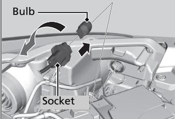
1. Turn the socket to the left and remove it.
