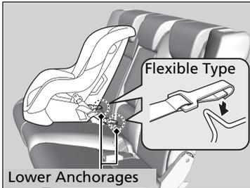
4. Place the child restraint system on the vehicle seat then attach the child restraint system to the lower anchorages according to the instructions that came with the child restraint system.
