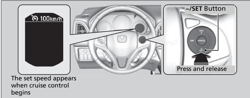
Take your foot off the accelerator pedal and press the **-/SET** button when you reach the desired speed.
