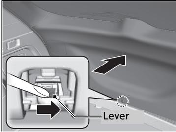
3. To open the tailgate, push the tailgate while sliding the lever to the right.
