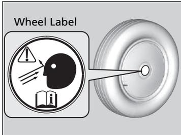
13. Apply the wheel label to the flat surface of the wheel.
