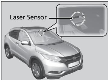
The City-Brake Active system unit, including the laser sensor, is located behind the rearview mirror.
