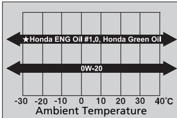
Use a commercial engine oil of suitable viscosity for the ambient temperature as shown.
