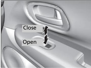
**To open:** Push the switch down lightly, and hold it until the desired position is reached.
