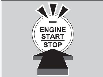
2. Depress the brake pedal (continuously variable transmission) or clutch pedal (manual transmission) and press the **ENGINE START/STOP** button within 10 seconds after the beeper sounds and the indicator stays on.
