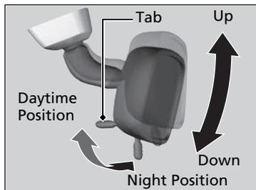
Flip the tab to switch the position. The night position helps to reduce the glare from headlights behind you when driving after dark.
