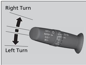
The turn signals can be used when the ignition switch is in ON **II**\*1.
