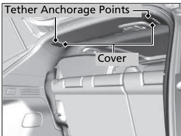
Two tether anchorage points are provided on the ceiling for rear outer seating positions. A child restraint system that is installed with a seat belt and comes with a tether can use the tether for additional security.
