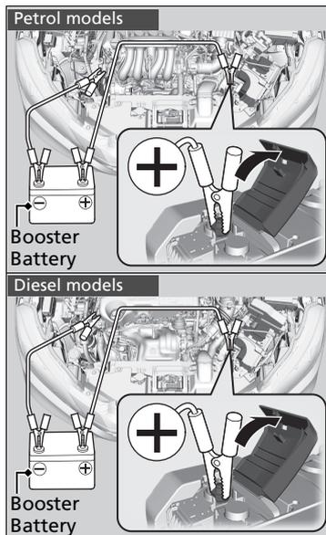
1. Connect the first jumper cable to your vehicle's battery  $\oplus$  terminal.
