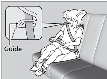
A back-rest is available for a specific booster seat. Install the back-rest to the booster seat and adjust it to the vehicle seat according to the booster seat manufacturer's instructions. Make sure the seat belt is properly routed through the guide at the shoulder of the back-rest and the belt does not touch and cross the child's neck.
