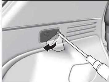
1. Pry on the edge of the light using a flat-tip screwdriver to remove the light assembly.
