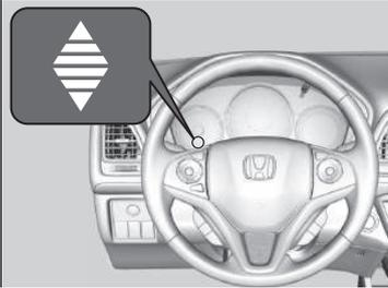
Come on while the vehicle is in the 7-speed manual shift mode to indicate when a speed change is appropriate to maintain the most fuel efficient driving style.
