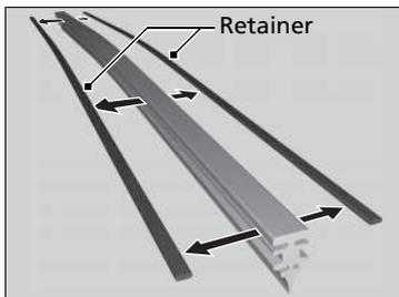
**4.** Remove the retainers from the rubber blade that has been removed, and mount to a new rubber blade.
