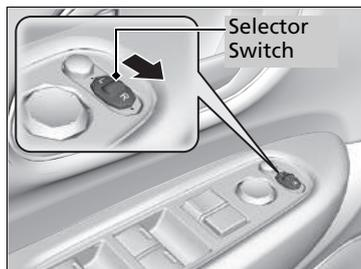
If activated, passenger side door mirror automatically tilts downward when you put the shift lever in **[R]**; this improves close-in visibility on the passenger side of the vehicle when reversing. The mirror automatically returns to its original position when you shift out of **[R]**.
