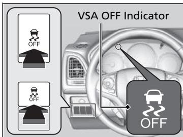
This button is on the driver side control panel. To partially turn the VSA features on and off, press and hold it until you hear a beep.
