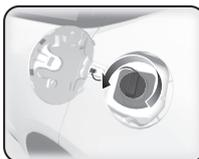
**3** Place the cap in the holder on the fuel fill door.
