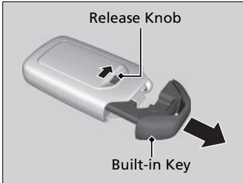
The built-in key can be used to lock the doors when the keyless remote battery becomes weak and the power door lock/unlock operation is disabled.
