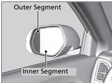
The driver's side door mirror has outer and inner segments. The outer segment is slightly curved to provide a wider angle view than a standard flat mirror. This wider view may help you check areas that are not visible using a standard door mirror.
