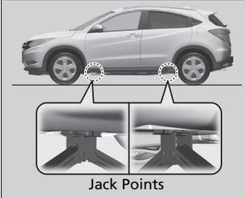
1. Place the jack under the jacking point closest to the tyre to be changed.
