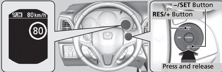
On when the intelligent speed limiter is set to the speed limit that the traffic sign recognition system detects.
