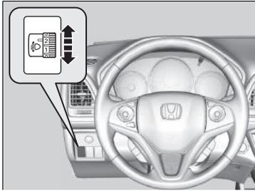
You can adjust the vertical angle of the low beam headlights when the ignition switch is in ON
