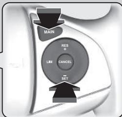
If a different indicator comes on, press the **LIM** button to switch the cruise control.
