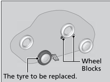
5. Place a wheel block or rock in front and rear of the wheel diagonal to the flat tyre.
