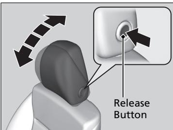
**To tilt the head restraint forward:** Push the back of it forward.
