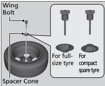
2. Remove the spacer cone from the wing bolt, flip it over, and insert it back on the bolt.
