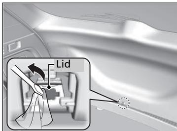
2. Wrap a cloth around the flat-tip screwdriver. Put it into the lid as shown in the image, and open the lid.
