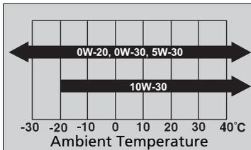
Use a Genuine Honda Motor oil or another commercial engine oil of suitable SAE viscosity for the ambient temperature as shown.
