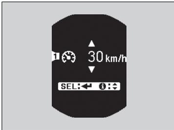
1. Press the button until the speed alarm setting menu appears on the display, then press the **SEL/RESET** button.
