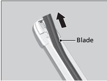
**3.** Slide the wiper blade out from its holder by pulling the tabbed end out.
