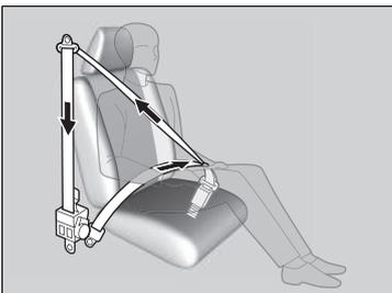
The tensioners automatically tighten the front and rear outer seat belts during a moderate-to-severe frontal collision, sometimes even if the collision is not severe enough to inflate the front airbags.
