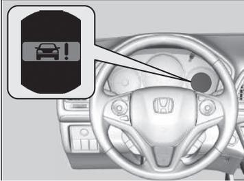
The beeper sounds, and a
