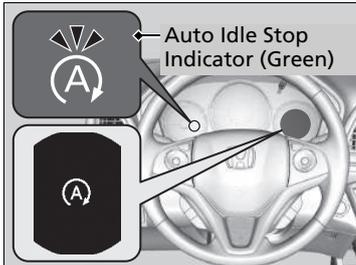
The engine then restarts once the vehicle is about to move again when you depress the clutch pedal, and the indicator (green) goes off.
