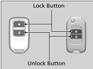
**To open:** Press the unlock button twice within 10 seconds and hold it down for the second time.
