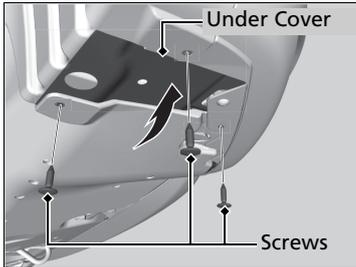
1. Remove the screws using a Phillips-head screwdriver, then push up the under cover.
