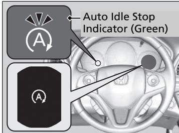
The engine then restarts once the vehicle is about to move again, and the indicator (green) goes off.
