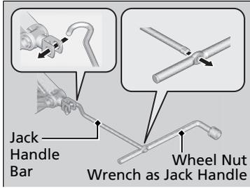
3. Raise the vehicle, using the jack handle bar and the jack handle, until the tyre is off the ground.
