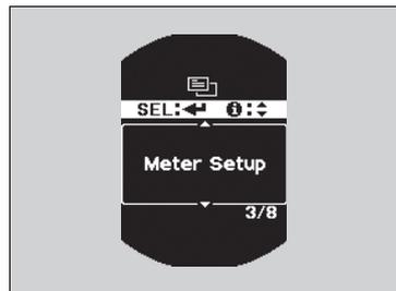
2. Press the button until **Meter Setup** appears on the display.
