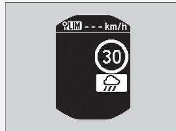
■ **When the traffic sign recognition system detects the speed limit sign while the intelligent speed limiter is paused**
