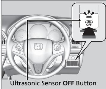
To turn off the ultrasonic sensor system, press the ultrasonic sensor **OFF** button after you remove the key from the ignition switch, or with the key in the ACCESSORY **I** or LOCK **0**\*1.
