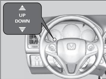
Come on to indicate when a gear change is appropriate to maintain the most fuel efficient driving style.
