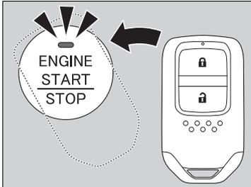
1. Touch the centre of the **ENGINE START/STOP** button with the **H** logo on the keyless remote while the indicator on the **ENGINE START/STOP** button is blinking. The buttons on the keyless remote should be facing you.
