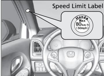
1. Apply the speed limit label to the location as shown.
