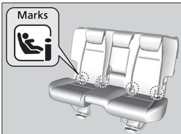
1. Locate the lower anchorages under the marks.
