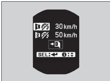
1. Press the /▼ button until the speed alarm setting screen appears on the display, then press the **SEL/RESET** button.
