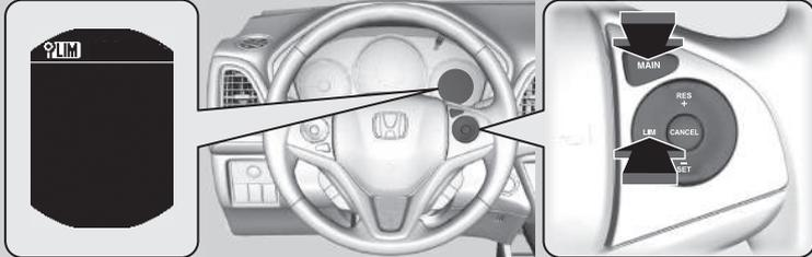
If a different indicator comes on, press the **LIM** button to change it to the intelligent speed limiter.
