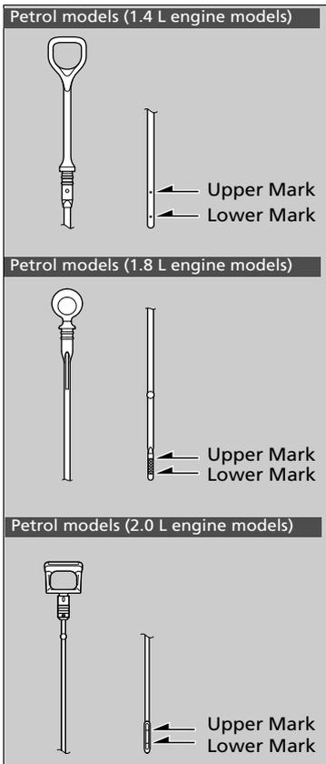
4. Remove the dipstick again, and check the level. It should be between the upper and lower marks. Add oil if necessary.
