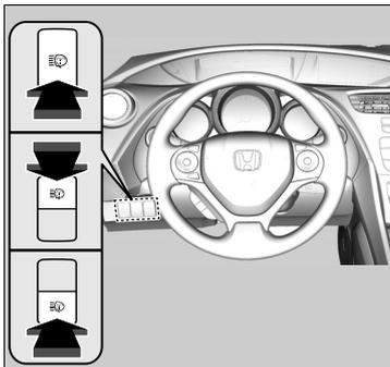
Turn the headlights on and press the headlight washers button to operate. The headlight washers also operate when you turn the windscreen washers for the first time after the ignition switch is turned to ON **II**\*1.
