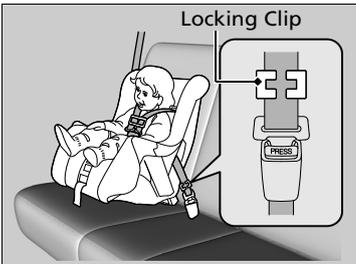
3. Tightly grasp the belt near the latch plate. Pinch both parts of the belt together so they do not slip through the latch plate. Unbuckle the seat belt.
