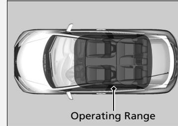
You can start the engine when the keyless remote is inside the vehicle. The engine may also run if the keyless remote is close to a door or window, even if it is outside the vehicle.
