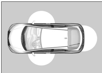
When you carry the keyless remote, you can lock/unlock the doors and open the tailgate.
