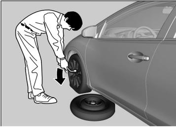
**11.** Loosen each wheel nut about one turn using the wheel nut wrench.
