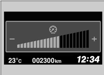
When the ignition switch is in ON
