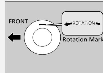
When the tyres are rotated, make sure the air pressures are checked.
