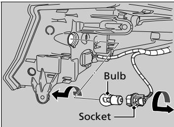
5. Turn the socket to the left and remove it.
