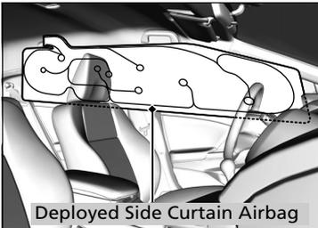
The side curtain airbag is designed to deploy in a moderate-to-severe side impact.
