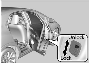
Slide the lever in the rear door to the lock position, and close the door.
