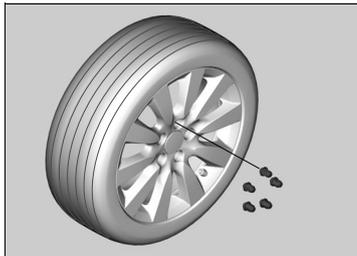
1. Remove the wheel nuts and flat tyre.
