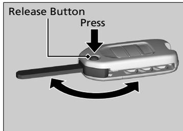
The key folds up inside the remote transmitter.
