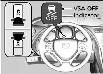
This button is on the driver side control panel. To turn the VSA system on and off, press and hold it until you hear a beep.
