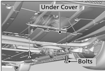
1. Remove the bolts, then remove the under cover.
