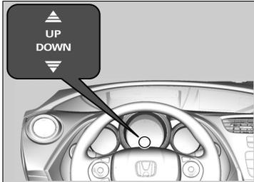
Come on to indicate when a gear change is appropriate to maintain the most fuel efficient driving style.
