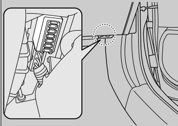
Fuse locations are shown on the image. Locate the fuse in question by the fuse number in the image and chart.
