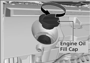
1. Unscrew and remove the engine oil fill cap.
