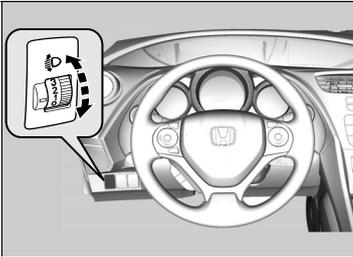
You can adjust the vertical angle of the low beam headlights when the ignition switch is in ON **II**\*1.
