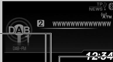
The DAB indicator appears on the display when the DAB band is selected.
