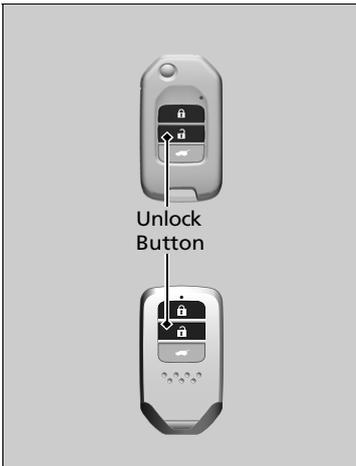
**To open:** Press the unlock button twice within 10 seconds and hold it down for the second time.
