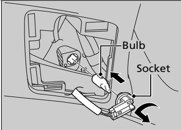
2. Turn the socket to the left and remove it.
