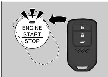
1. Touch the centre of the **ENGINE START/STOP** button with the **H** logo on the keyless remote while the indicator on the **ENGINE START/STOP** button is blinking. The buttons on the keyless remote should be facing you.
