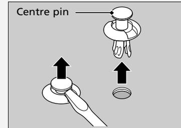
Insert the clip with the central pin raised, and push until it is flat.
