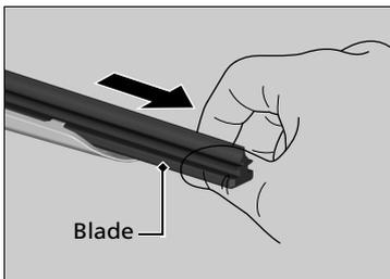
4. Slide the wiper blade out from its holder by pulling the tabbed end out.
