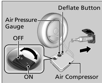
4. Turn on the air compressor and inflate the tyre to the required air pressure.
