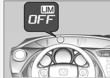
If there is a problem with the system when you are using the adjustable speed limiter, the beeper sounds and **OFF** comes on. The adjustable speed limiter will be turned off.
