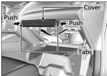
5. Push in the tabs on the corners of the filter case cover, and remove it.
