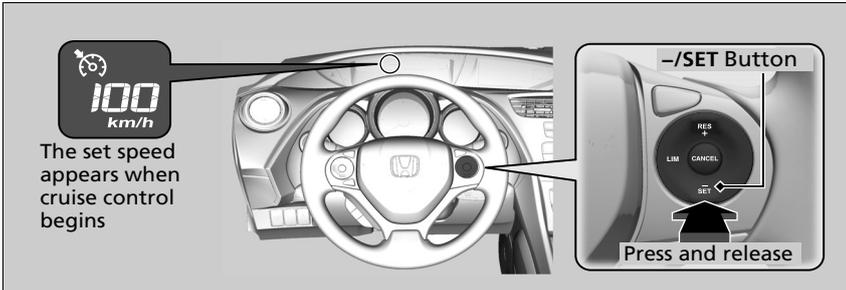
Take your foot off the accelerator pedal and press the **-/SET** button when you reach the desired speed.
