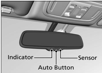
Reduces the glare from headlights behind you when driving after dark. Press the auto button to turn this function on and off. When activated, the auto indicator comes on.
