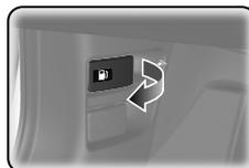
**2** Turn the fuel fill cap slowly to remove the cap.
