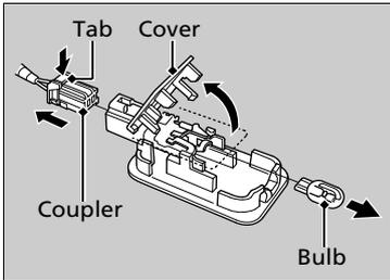
2. Push the tab to remove the coupler.
