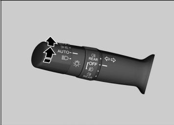
Automatic lighting control can be used when the ignition switch is in ON
