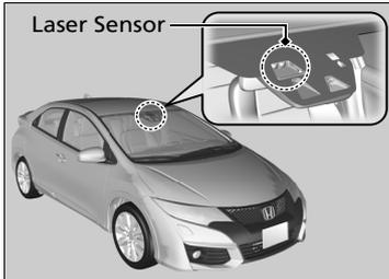
The City-Brake Active system unit, including the laser sensor, is located behind the rearview mirror.
