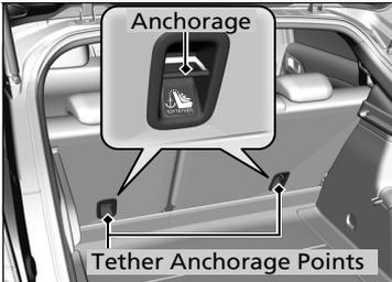
A tether anchorage point is provided behind each rear outer seating position. A child restraint system that is installed with a seat belt and comes with a tether can use the tether for additional security.
