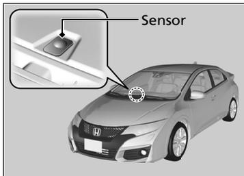
The automatic climate control system is equipped with sensors. Do not cover or spill any liquid on them.
