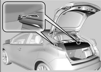
3. Pull the cover towards you until it disengages from the support rods, and lift it up to remove.
