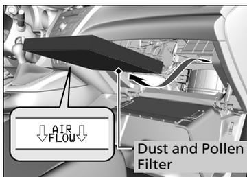
6. Remove the filter from the case.
