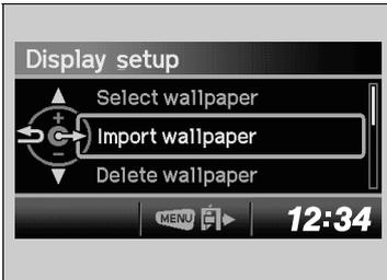
5. Select **Import wallpaper** with the  $\left[ \begin{smallmatrix} + \\ - \end{smallmatrix} \right]$  /  $\left[ \begin{smallmatrix} \leftarrow \\ \rightarrow \end{smallmatrix} \right]$  button, then press the **SOURCE** button.
