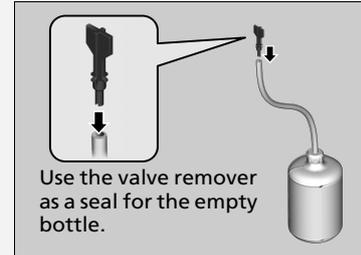
Keep the empty bottle after the sealant is injected. The sealant bottle will be used to collect the injected sealant by a professional.
