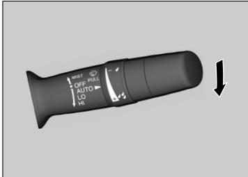
When you push the lever down to **AUTO**, the windscreen wipers sweep once, and go into the automatic mode.
