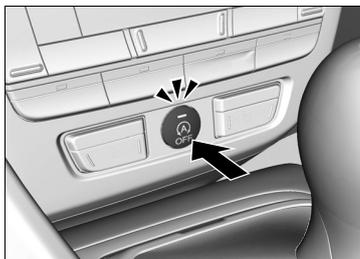
To turn the Auto Idle Stop system off, press this button. The Auto Idle Stop system stops.
