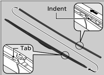
6. Slide the new wiper blade onto the holder from the bottom end.
