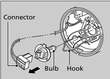
2. Unhook the hook, and pull out the connector.
