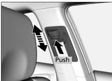
1. Move the anchor up and down while holding the release button.
