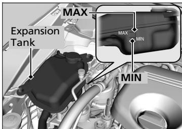
1. Check the amount of coolant in the expansion tank.
