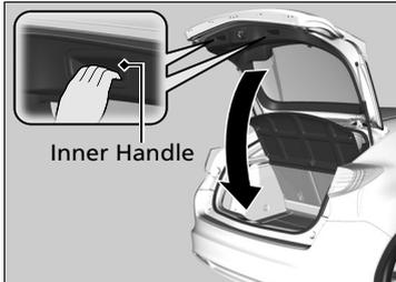
To close the tailgate, grab the inner handle, pull the tailgate down, and push it closed from outside.
