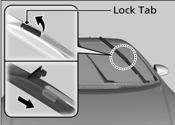
2. Place a cloth on the edge of the lock tab. Push the lock tab up with a flat-tip screw driver.
