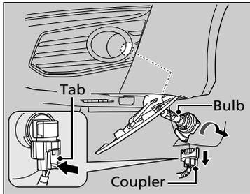
3. Push the tab to remove the coupler.
