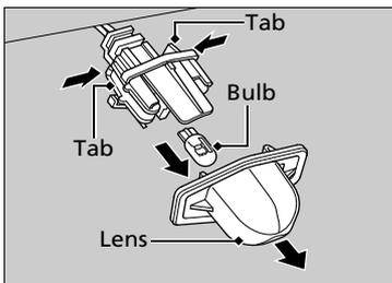
**2.** Remove the lens by pushing the tabs.
