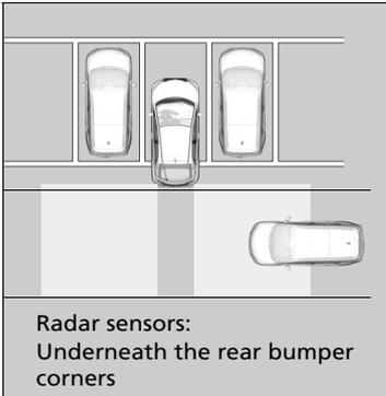
When a vehicle approaches from a rear corner, cross traffic monitor alerts you with a buzzer and a displayed warning.
