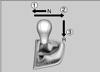
1. Depress the clutch pedal, move the shift lever all the way to the left, and shift to **R**.
