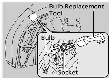
3. Turn the socket to the left and remove it.
