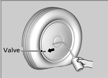
6. Screw the filler tube onto the tyre valve.
