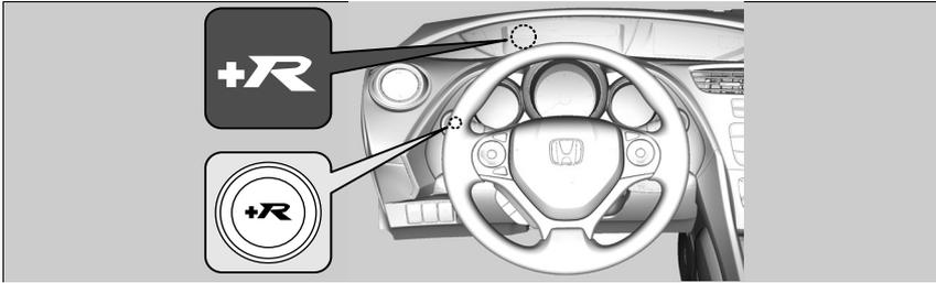
The **+R** button turns the +R mode on and off.
