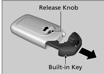
The built-in key can be used to lock/unlock the doors and tailgate when the keyless remote battery becomes weak and the power door lock/unlock operation is disabled. To remove the built-in key, pull it out while sliding the release knob. To reinstall the built-in key, push the built-in key into the keyless remote until it clicks.
