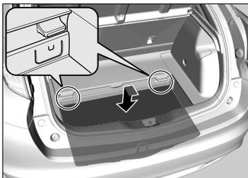
3. Push the far end of the lid down to the bottom of the under-floor storage area, then lower the other end.
