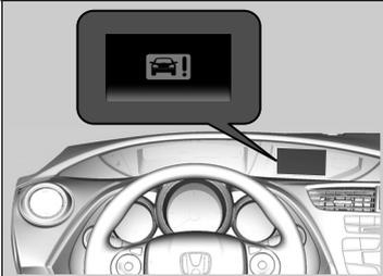
The beeper sounds, and a CTBA warning blinks on the i-multi-information display, and hard braking is applied when a possible collision becomes likely unavoidable.
