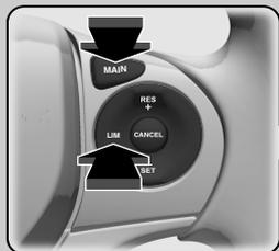
If a different indicator comes on, press the **LIM** button to switch the cruise control.
