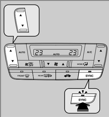
You can set the temperature synchronously for the driver side and the passenger side in synchronized mode.
