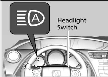
Turn the headlight switch in **AUTO** and pull the headlight lever to low beam.
