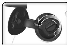
**3** Place the cap in the holder on the fuel fill door.
