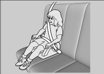
If a lap/shoulder seat belt cannot be used properly, position the child in a booster seat in a rear seating position. For the child's safety, check that the child meets the booster seat manufacturer's recommendations.
