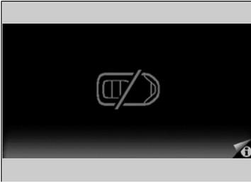
Warning buzzers may sound from inside or/ and outside the vehicle to remind you that the keyless remote is out of the vehicle. If the buzzer continues even after the remote is put back inside, place it to be within its operational range.
