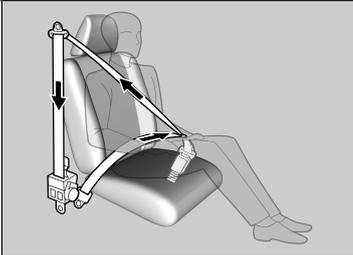
The front seats are equipped with automatic seat belt tensioners to enhance safety.
