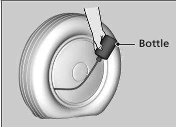
7. Hold the bottle upside down, and inject the sealant completely.
