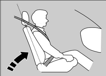
Adjust the driver's seat-back to a comfortable, upright position, leaving ample space between your chest and the airbag cover in the centre of the steering wheel.
