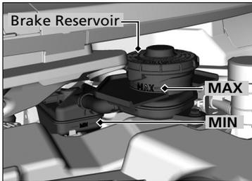
The fluid level should be between the **MIN** and **MAX** marks on the side of the reservoir.
