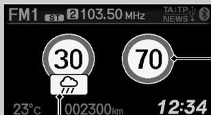
Additional Speed Limit Sign Based on Conditions\*2
