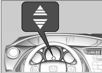
Come on while the vehicle is in the sequential shift mode to indicate when a gear change is appropriate to maintain the most fuel efficient driving style.
