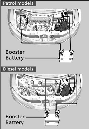
1. Connect the first jumper cable to your vehicle's battery  $\oplus$  terminal.
