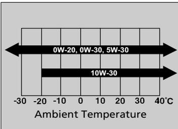
Use a Genuine Honda Motor oil or another commercial engine oil of suitable SAE viscosity for the ambient temperature as shown.
