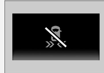
Indicates in amber that the rear bumper corners are covered with snow, mud, etc. The system is temporarily cancelled. Remove debris from the rear bumper corners.
