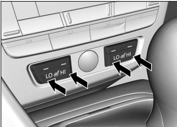
The indicator for your setting comes on while the seat heater is in use. Briefly press the button on the opposite side to turn the heater off. The indicator goes off. While in **HI**, the heater cycles on and off. When a comfortable temperature is reached, select **LO** to keep the seat warm.
