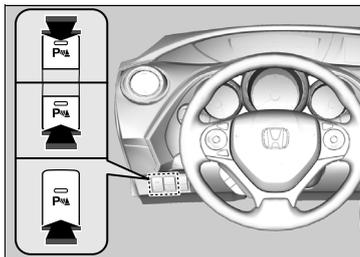
With the ignition switch in ON **[II]**\*1, press the parking sensor system button to turn on or off the system. The indicator in the button comes on when the system is on.
