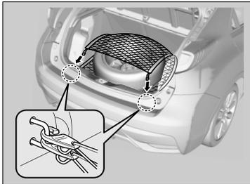
4. Wrap the flat tyre with the net, then attach the other two hooks to the same luggage hooks as shown.
