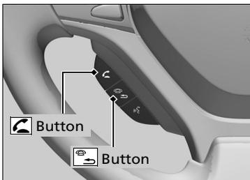
Press the (pick-up) button on the steering wheel to receive a call when *Bluetooth*® Audio is playing.
