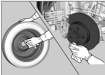
2. Wipe the mounting surfaces of the wheel with a clean cloth.
