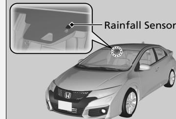
Do not put the wiper lever in **AUTO** when cleaning the windscreen or driving through a car wash. If the wiper lever is in **AUTO**, and the ignition switch is in ON **II**<sup>\*1</sup>, the rainfall sensor may respond to your hand or car wash liquids, and the wipers may operate automatically.
