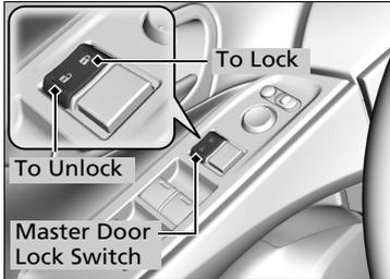
Press the master door lock switch in as shown to lock or unlock all doors and the tailgate.
