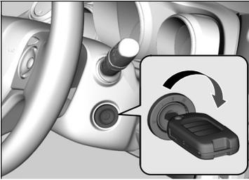
3. Turn the ignition switch to START
