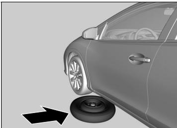
10. Place the spare tyre (wheel side up) under the vehicle body, near the tyre that needs to be replaced.
