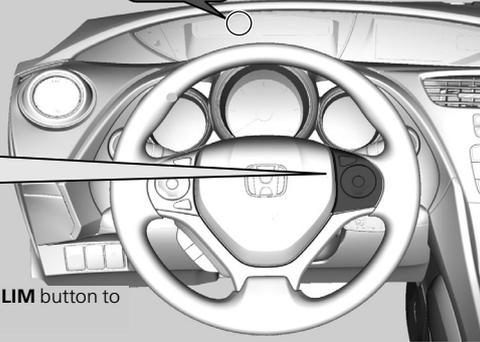
If a different indicator comes on, press the **LIM** button to switch to the adjustable speed limiter.
