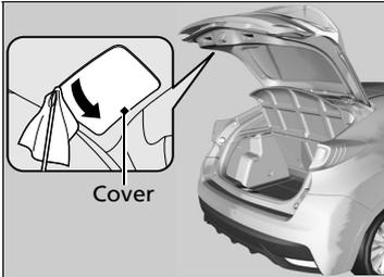
1. Pry on the edge of the cover using a flat-tip screwdriver to remove it.
