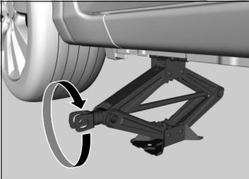
2. Turn the end bracket clockwise as shown in the image until the top of the jack contacts the jacking point.
