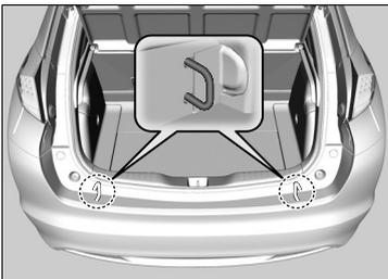
The luggage hooks in the luggage area can be used to install a net for securing items.
