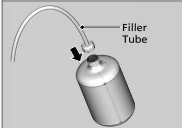
2. Screw the filler tube onto the bottle.
