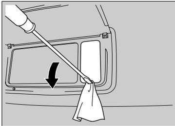
1. Pry on the edge of the cover using a flat-tip screwdriver to remove the cover.
