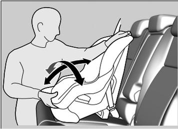
6. Make sure the child restraint system is firmly secured by rocking it forward and back and side to side; little movement should be felt.
