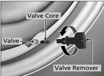
5. Unscrew the valve core using the valve remover. Do not place the valve core in sand or dirt.
