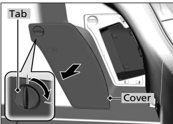
Turn and pull the tab to open the compartment cover located on the side of the luggage area.
