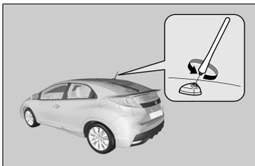
Your vehicle is equipped with a removable antenna at the rear of the roof.
