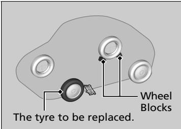
9. Place a wheel block or rock in front and rear of the wheel diagonal to the flat tyre.
