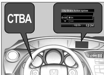
You can turn the system on and off using the i-multi-information display.
