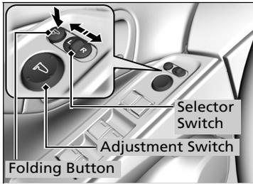
You can adjust the door mirrors when the ignition switch is in ON
