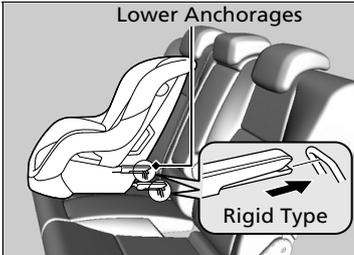
1. Locate the lower anchorages under the marks.
