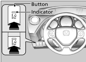
Press the Lane Departure Warning button to turn the system on and off.
