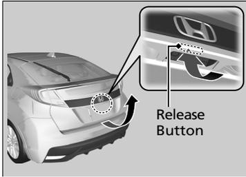
When all the doors are unlocked or the tailgate unlock button on the remote transmitter is pressed, the tailgate is unlocked. Press the tailgate release button and lift open the tailgate.
