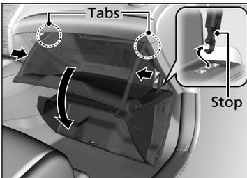
2. Push the stop on the passenger's side of the glove box to detach it from the glove box.
