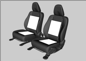
The ignition switch must be in ON **II**\*1 to use the seat heaters. The **HI** setting heats the seats faster than the **LO** setting.
