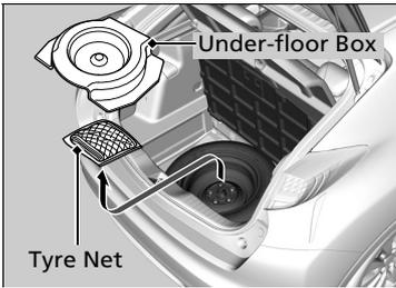
7. Remove the under-floor box, then take the tyre net out.
