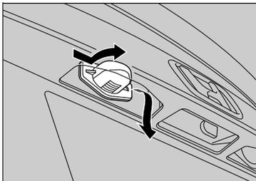
**1.** Remove the licence plate light assembly by pushing the left edge of the lens towards the right and pulling the assembly out.
