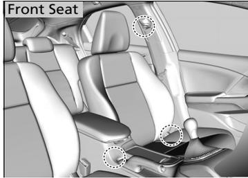
When replacing the seat belts, use the anchorage points shown in the images. The front seat has a lap/shoulder belt.
