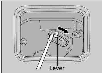
2. To open the tailgate, push the tailgate while pushing down the lever with the flat-tip screw driver.
