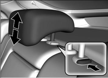
A passenger sitting in a back seating position should adjust the height of their head restraint to an appropriate position before the vehicle begins moving.
