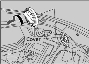
1. Rotate the cover to the left and remove it.
