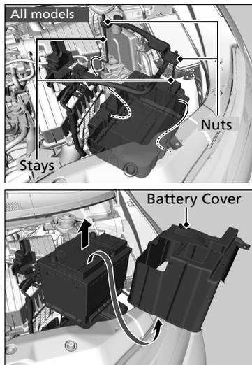
5. Loosen the nut on each side of the battery bracket with a wrench.
