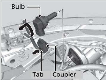
1. Push the tab to remove the coupler.
