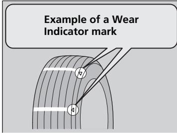
The groove where the wear indicator is located is 1.6 mm (1/16 inch) shallower than elsewhere on the tyre. If the tread has worn so that the indicator is exposed, replace the tyre.
