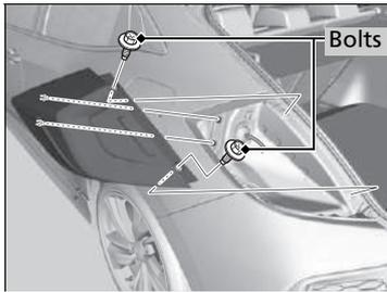
1. Use a Phillip-head screwdriver or socket to remove the bolts.
