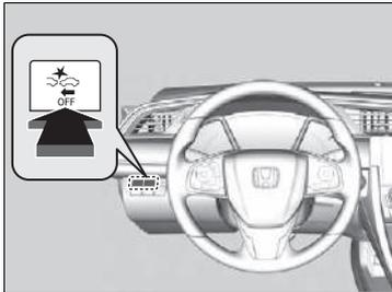
Press and hold the button until the beeper sounds to switch the system on or off.
