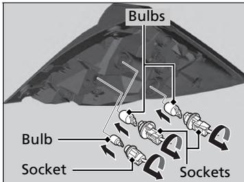
3. Turn the socket anticlockwise and remove it.
