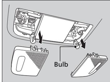
3. Remove the old bulb and insert a new bulb.
