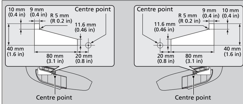
1. Prepare for two rectangular pieces of masking tape, measuring 40 mm (1.6 in) wide and 80 mm (3.1 in) long.
