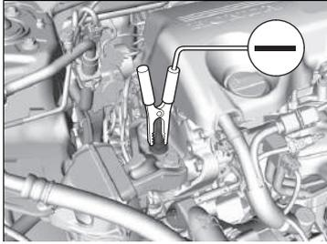
5. Connect the other end of the second jumper cable to the engine mounting bolt as shown. Do not connect this jumper cable to any other part.
