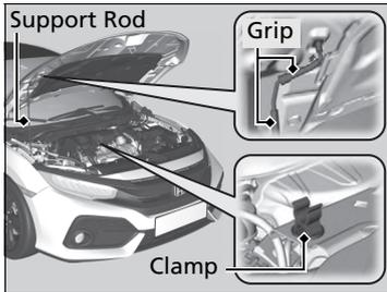
4. Remove the support rod from the clamp using the grip. Mount the support rod in the bonnet.
