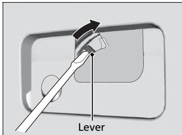
**2.** To open the hatch, push the hatch while sliding the lever with the flat-tip screw driver.
