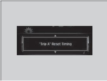
4. Press the
