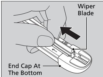
3. Pull the end of the wiper blade in the direction of the arrow in the image until it is out of the holder's end cap.
