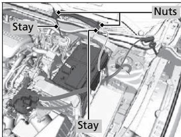
4. Loosen the nut on each side of the battery bracket with a wrench.
