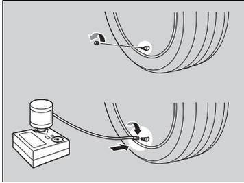
4. Recheck the air pressure using the gauge on the air compressor.
