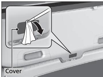
**1.** Remove the cover on the back of the hatch by prying it off with a small flat-tip screwdriver.
