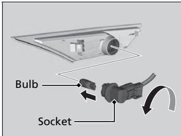
3. Turn the socket anticlockwise to remove it, then remove the old bulb.
