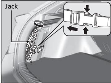
3. Turn the jack's end bracket to loosen it, then remove it.
