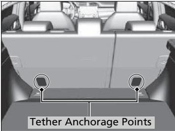
Two tether anchorage points are located behind each rear outer seating positions. If you have a child restraint system that comes with a tether but can be installed with a seat belt, the tether may be used for additional security.
