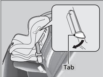
1. Place the child restraint system on the vehicle seat.
