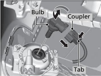
2. Push the tab to remove the coupler.
