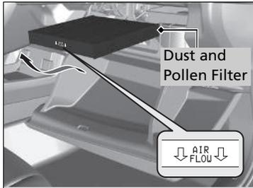
6. Remove the filter from the case.
