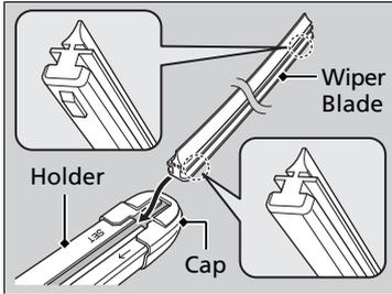
**5.** Insert the flat side of the new wiper blade onto the bottom part of the holder. Insert the blade all the way.
