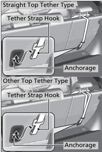
2. Raise the head restraint to its highest position, then route the tether strap between the head restraint legs, and secure the tether strap hook to the anchorage.
