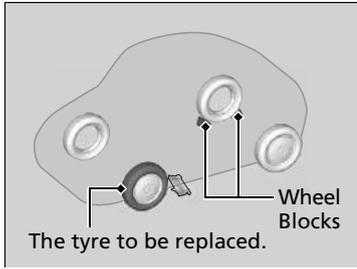
6. Place a wheel block or rock in front and rear of the wheel diagonal to the flat tyre.
