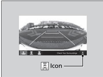
Tap to turn the system on and off. The indicator (green) comes on with the system on.
