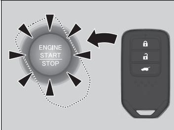
1. Touch the centre of the **ENGINE START/STOP** button with the **H** logo on the keyless remote while the **ENGINE START/STOP** button is flashing. The buttons on the keyless remote should be facing you.
