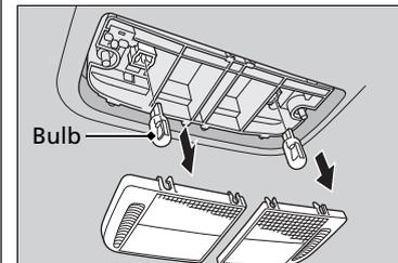
3. Remove the old bulb and insert a new bulb.
