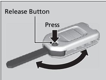
The key folds up inside the remote transmitter.
