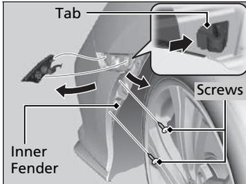
1. Remove the screws, and pull the inner fender back.
