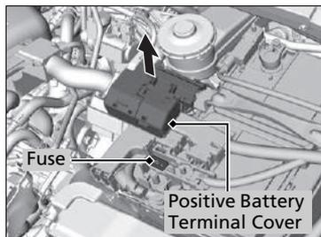
Remove the cover on the ⊕ terminal (as shown).
