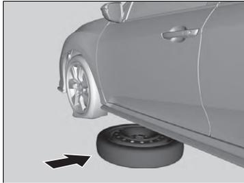
7. Place the spare tyre (wheel side up) under the vehicle body, near the tyre that needs to be replaced.
