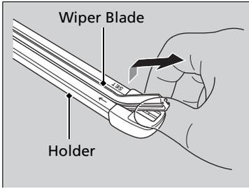
**4.** Pull the wiper blade in the opposite direction to slide it out of holder.
