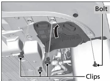
1. Remove the clips using a flat-tip screwdriver, remove the bolt, and push up the under cover.
