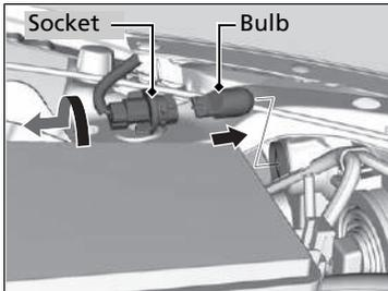
1. Turn the socket anticlockwise and remove it.
