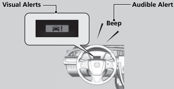
At system's earliest collision alert stage, you can change the distance (**Far/Normal/Near**) between vehicles at which alerts will come on through driver information interface or audio/information screen setting options.
