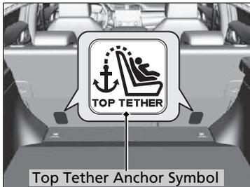
3. Place the child restraint system on the vehicle seat, then attach the child restraint system to the lower anchorages according to the instructions that came with the child restraint system.
