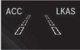
When the LKAS is suspended, the lane lines on the driver information interface change to contour lines, and the beeper sounds (if activated).
