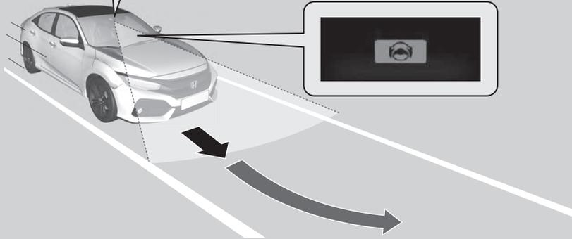
When you operate the turn signals to change lanes, the system is suspended, and resumes after the signals are off.
