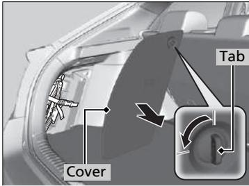
2. Turn and pull the tab to open the compartment cover located on the left side of the luggage area.
