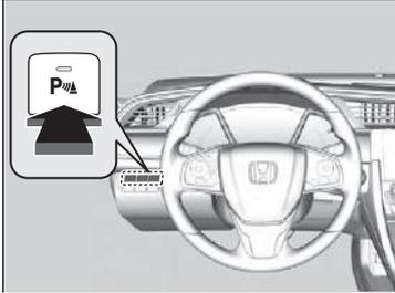
With the ignition switch in ON **[II]**\*1, press the parking sensor system button to turn on or off the system. The indicator in the button comes on when the system is on.
