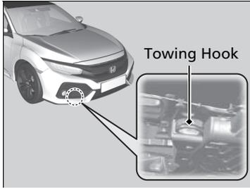
1. Hook the towing device to the towing hook.
