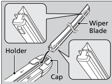
7. Insert the flat side of the new wiper blade onto the bottom part of the holder. Insert the blade all the way.
