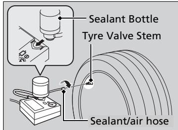
1. Remove the valve cap from the tyre valve stem.
