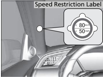
1. Apply the speed restriction label to the location as shown.
