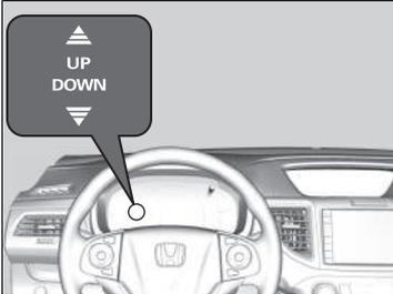
Come on while the vehicle is in the sequential mode to indicate when a gear change is appropriate to maintain the most fuel efficient driving style.
