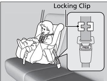
3. Tightly grasp the belt near the latch plate. Pinch both parts of the belt together so they do not slip through the latch plate. Unbuckle the seat belt.
