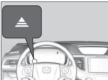
Come on while the vehicle is in the sequential shift mode to indicate when a gear change is appropriate to maintain the most fuel efficient driving style.
