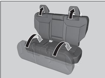
2. Push the head restraint up to its original position.
