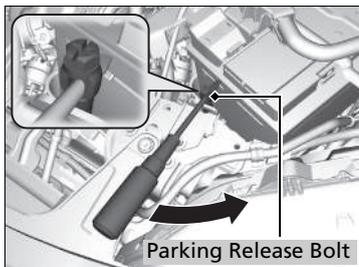
4. Insert a screwdriver into the hole in the shaft of the parking release bolt. Swing the screwdriver anticlockwise to loosen the parking release bolt.
