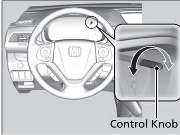
When the position lights are turned on and the ignition switch is in ON
