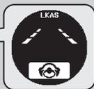
When you operate the turn signals to change lanes, the system is suspended, and resumes after the signals are off.
