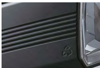
Front grille parts made of "recycled bumper material"
